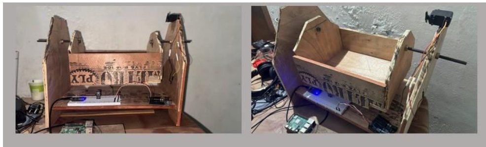
Figure 6.2: Cradle setup with sensors and Raspberry Pi
